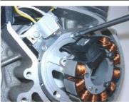
Put the base plate (consisting of the outer steel ring and the inner aluminium plate) into the place of your old generator.
