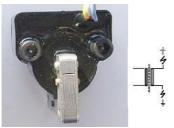
Typical resistance between both exits is 6.2kOhm. Both exists fire at the same time (as many twin systems do). Sparks will be polarised however at a 180 degrees difference which might manifest when you strobe it.
