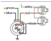
Disconnect all cables from your old generator, regulator and the ignition coils and remove those parts. You may pull your old rotor from the crankshaft by means of a puller screw M8x90.
