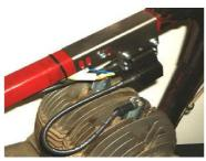
Fasten the new ignition coil at the place the old coils have been. We provide some holder with screws that should enable you to fit the coil there. To use this, fit the coil with its HT exits facing backwards (towards the seat). Unfortunately the stock coil fastening hole in the frame seems to have been drilled at random, so our holder will not always fit without modification, even though we have provided oblong holes.
